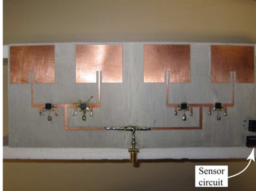
Fig. 12. Picture of the manufactured 1 \times 4 SELFLEX array prototype ( g = 2.0 mm, h = 35.6 mm, m = 19.8 mm, s = 11.0 mm, t = 1.3 mm, u = 33.4 mm, and w = 43.6 mm).
